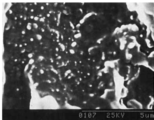
Figure 12 SEM photograph of PEA(H)/PPY composite (cross-section).
